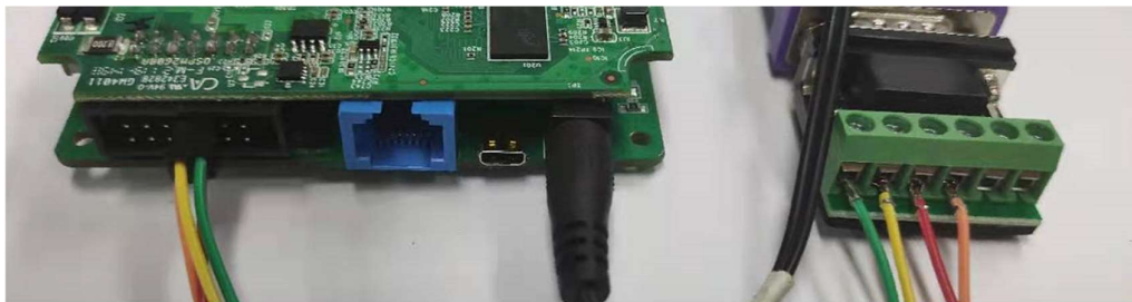
Figure 19: RS422 connection diagram
